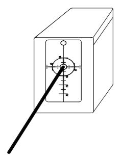
The safety photoelectric device DFS LASER is a mono-ray barrier with visible laser emission that, integrated in a more general check system, contributes to the operator's protection when using machines having movable dangerous parts, controlled by electrical or electromechanical devices.
